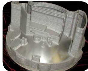
Defense Housing Fabricated by LENS System
