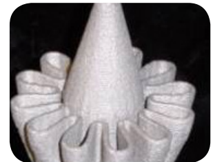
Exhaust Duct Fabricated by LENS System
