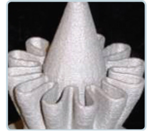
Exhaust Duct Fabricated by LENS System
