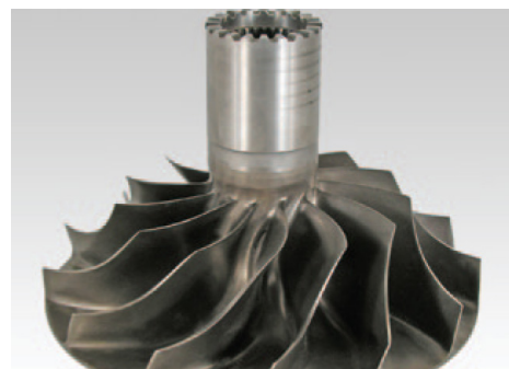
Impeller repaired by LENS 1500 AM CA System
