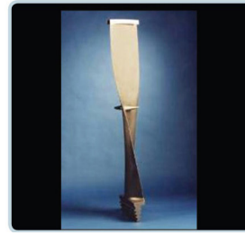
Compressor Blade Repaired by LENS System
