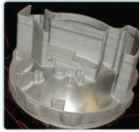
Defense Housing Fabricated by LENS/CNC Process
